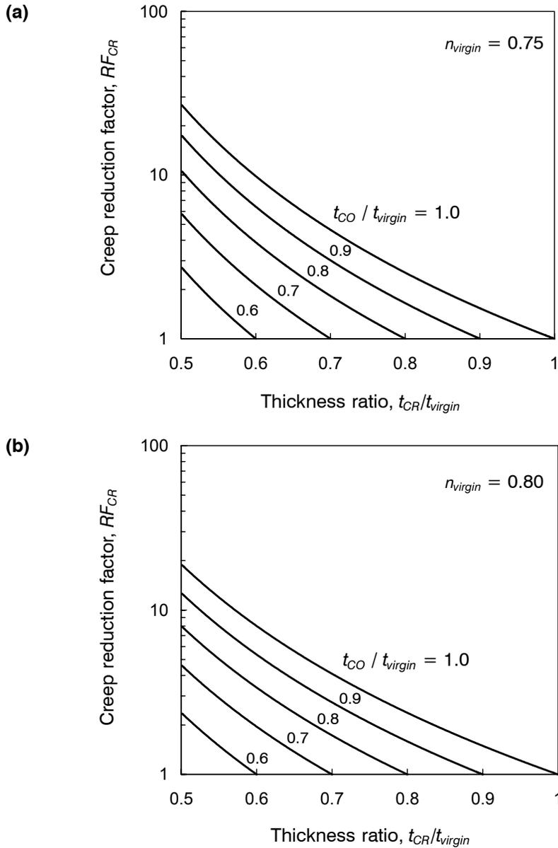
**Figure 5.** Value of the hydraulic transmissivity reduction factor due to creep (“creep reduction factor”) as a function of the thickness ratios,  $t_{CO}/t_{virgin}$  and  $t_{CR}/t_{virgin}$ , for four values of the initial porosity: (a)  $n_{virgin} = 0.75$ ; (b)  $n_{virgin} = 0.80$  (Figure 5 continues on the next page).
