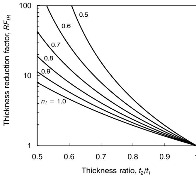
**Figure 4.** Value of the hydraulic transmissivity reduction factor due to thickness reduction as a function of the thickness ratio,  $t_2/t_1$ , and the geosynthetic porosity in the initial state,  $n_1$ .
